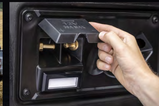
With the professional package option you will find two electrical 12V plug integrated into the fuel tank to power an external fuel or AdBlue® pump.
