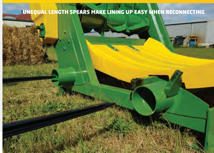
FORGED HAY SPEARS PIERCE THE BALE RATHER THAN PUSHING IT
