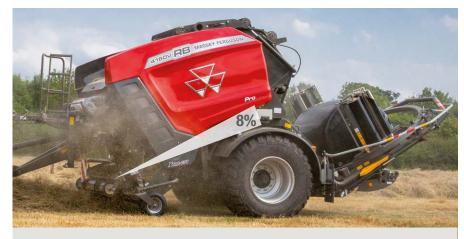
The new Protec combination unit has a lower crop elevation angle, reducing the overall baler height. This feature improves stability, allowing safer and faster hillside operation. It also reduces back pressure in the feeding area, streamlining crop flow and minimising the risk of blockages.
