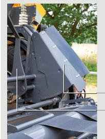
In addition to the transfer arm, the new design features two active guiding plates on both sides of the baler clearly directing the bale to the centre of the wrapper plate allowing for a faster and more secure transfer cycle. For added safety in hillside conditions the unique slope transfer mode allows for the transfer arm to move more slowly while the wrapper ring is lifted higher to receive the bale. This ensures that the bale will be securely delivered to the wrapper even in sloping terrain.
