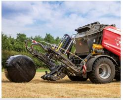
To ensure gentle bale unloading, the wrapping table is lowered close to the ground, thus minimising the bale's rolling speed, preventing film damage and maintaining the ideal bale shape. An optional bale tipper prevents bales rolling away and makes for easier trailer loading. The operator can also choose between automatic and manual unloading modes.
