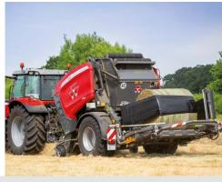
Once the bale is transferred to the centre of the wrapping table, a hydraulically driven wrapping ring begins to rotate before the tailgate is fully closed, completing the cycle well before the next bale is ready to wrap. Designed to withstand the heaviest bale loads, the robust frame and quiet running gear operates smoothly and effortlessly to wrap bale after bale.
