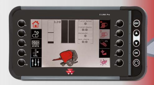
Specific field or customer information, such as the number of bales or hours worked, can easily be set and collected with the Wizard menu and later exported via USB connection for easy management of records and further performance analysis.
