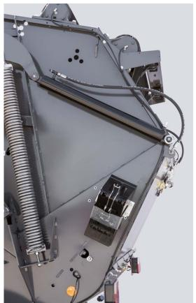
Bale volume increases exponentially in relation to its diameter, together with a corresponding belt pressure, to keep the bale density constant.
