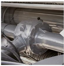
The Powersplit gearbox equally divides and transfers power to drive the rotor unit on one side and the roller drives on the other, reducing the overall power requirements by simplifying the drivelines. This results in a more efficient baler which uses less fuel.
