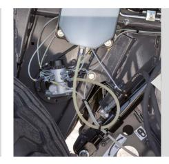
Automatic chain lubrication with individual adjustment for each chain guarantees sufficient oil supply, reduces maintenance time and extends chain service life. For added durability the highest quality chains are used throughout the baler.
