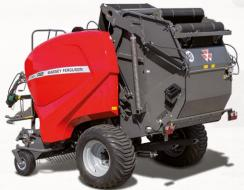
Massey Ferguson RB 4160V and RB 4180V round balers share a common platform and produce bales from 0.9m up to 1.60m or 1.80m in diameter respectively.
