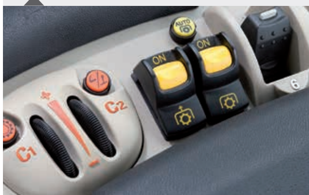
Command Centre PTO selector switches and Auto activation button.
