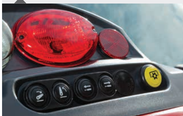
Fender mounted PTO, hydraulic spool valve and linkage controls.
