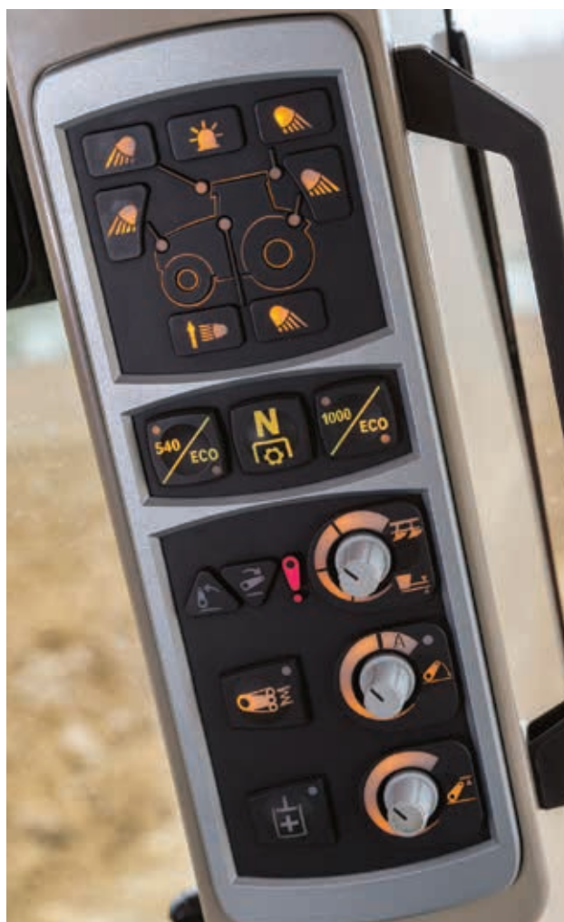
Pillar mounted PTO speed selection controls and linkage controls.
