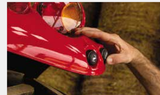
Fender mounted rear linkage controls
