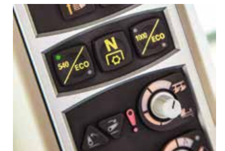
Electro-hydraulic PTO speed selection
