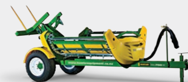
SL700X • Trailed, self-loading • 2 bale capacity • Up to 5 ft wide bales • Total Control Loading
