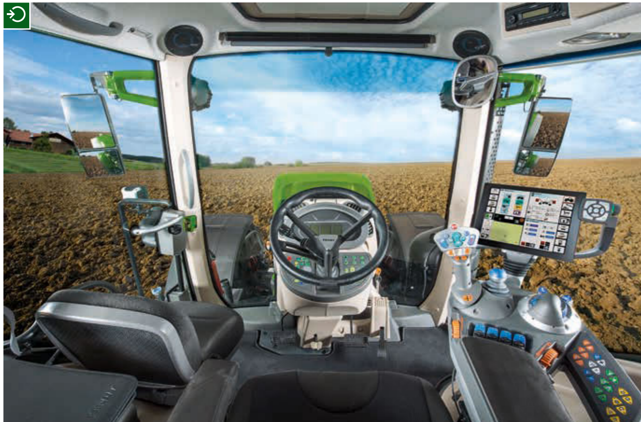
The 900 Vario has been trimmed for an optimal overview. The bonnet has been kept as narrow as possible, so drivers have an excellent view to the wheel arches and front-mounted implements.
