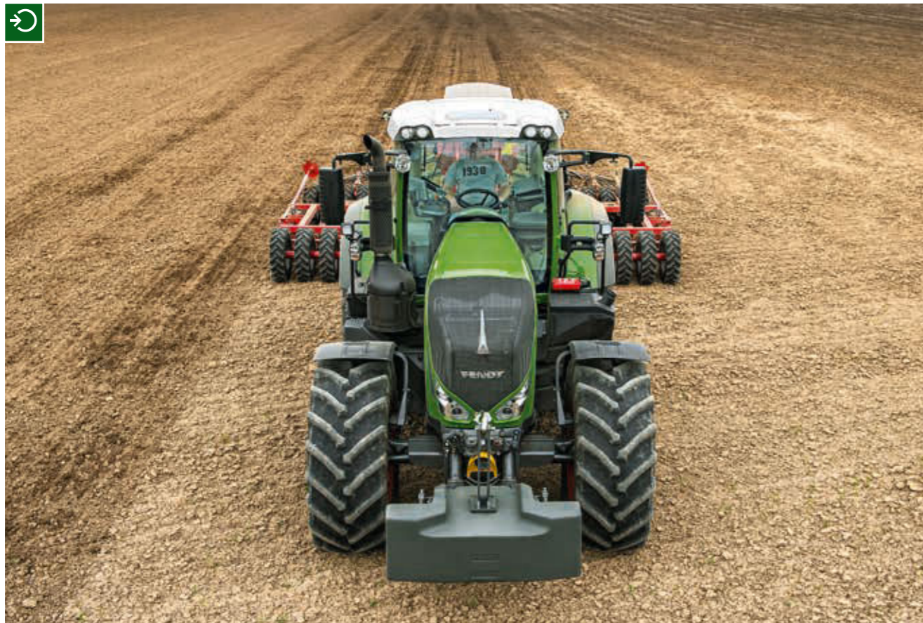
The Fendt 800 Vario has been trimmed for an optimal overview. The bonnet has been kept as narrow as possible, so drivers have an excellent view to the wheel arches and front-mounted implements.
