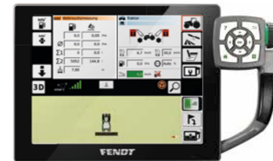
Always informed about everything – e.g. via the consumption indicator in the terminal.
