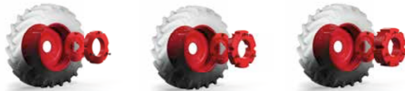
Wheel weights with 200 kg, 300 kg and 600 kg
