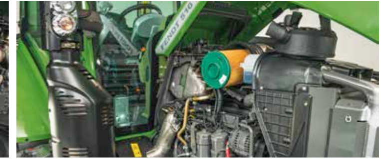
The air filter on the Fendt 500 Vario has a long life thanks to a precleaner and is easy to access for maintenance work.
