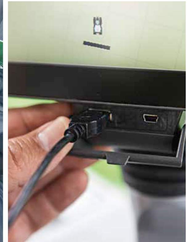
The field settings can be transferred to other Fendt tractors through the USB port. The port for charging mobile phones is also very practical.
