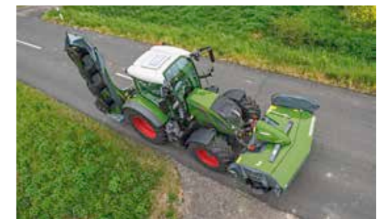
The Fendt 500 Vario reaches its final speed of 50 km/h at a low engine speed of 1700 rpm, 40 km/h already at 1400 rpm.
