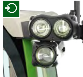
The crossed beams of the front work lights effectively prevent shadows.
