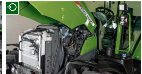
The fuel pre-filter with thermostatic valve allows the tractor to start reliably even at very low temperatures well below zero. The radiator and filter are arranged for ease of maintenance.
