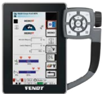
Display for crossgate lever and weighing system: individual and total weight and limiting of the working range for the arm and attachment.
