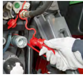
□ Power beyond pressure and control line for full hydraulic power transmission.
