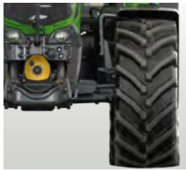
Large tyres of up to 540/65 R24 at the front and up to 600/65 R38 at the rear.
