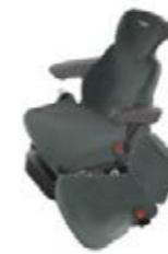
■ The comfort seat features air suspension and an easy-to-use armrest adjustment system.
