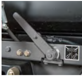
The lower links can be fixed with the shut-off valve on the rear linkage.
