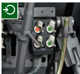
Both the DCUP and CUP couplings permit the hydraulic valves to be coupled under pressure and mounting and removing implements is easy. The self-closing valve flaps offer secure protection against contamination through dirt or water.
