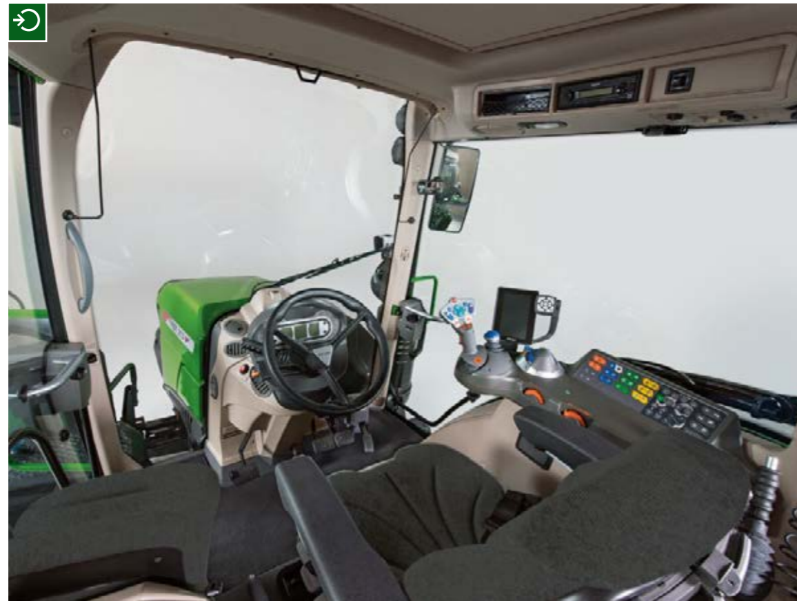
The clearly laid out and ergonomically designed VisioPlus cab offers the best overview, both to the operating elements and the field. The windscreen is available as a continuous panoramic window or as a hinged pane. An additional door can be chosen in place of the right side part.
