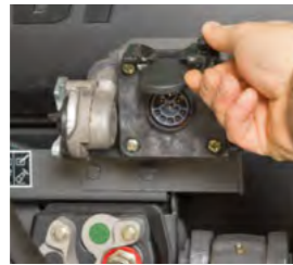
□ ISOBUS implement control connection.
