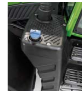
The Diesel and AdBlue filler necks are located on the same side of the tractor within easy reach from the ground.
