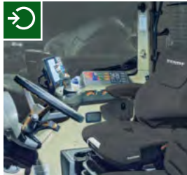
A light sensor automatically adapts the terminal lighting to the current light conditions.
