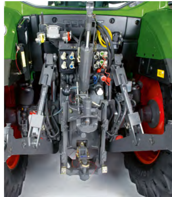
Interfaces at the rear include the signal socket, hydraulic top link, lower links with hooks, spool valves, free return, air brake, power beyond pressure and control lines, hydraulic trailer brakes, 7-pin socket, hitch, 540/540E/1000rpm rear PTOs, bottom hitch configuration, rigid drawbar and much more.
