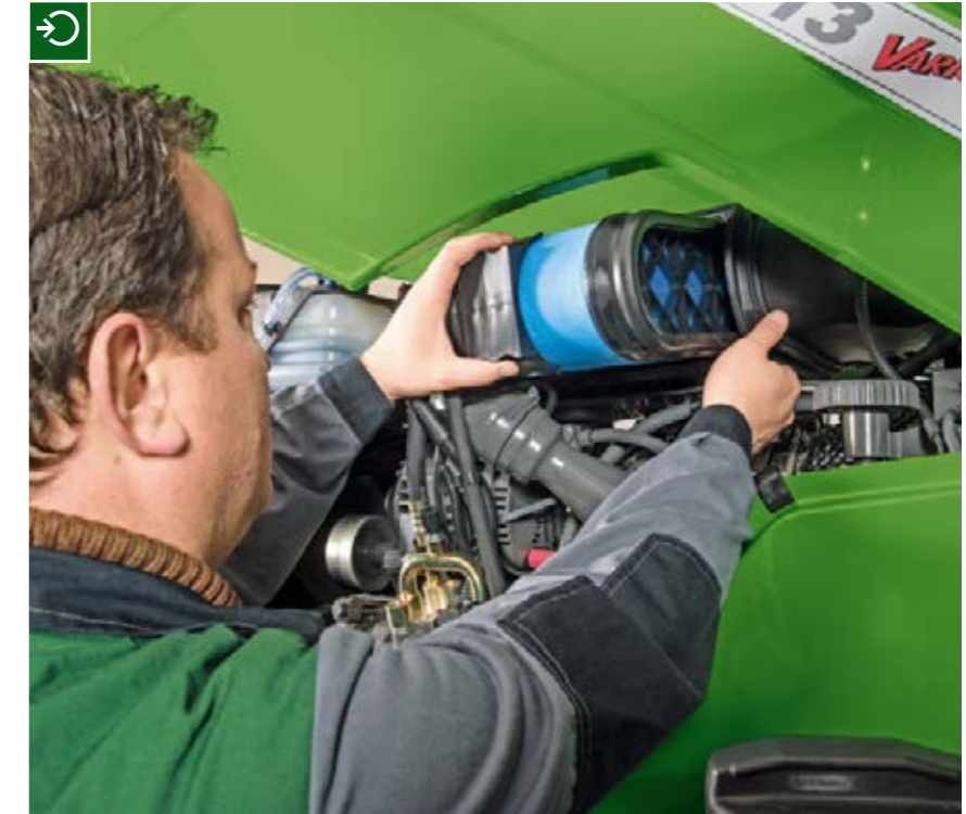
The high-capacity air filter ensures optimal air intake and cleaning. The air filter is easy to replace.
