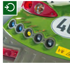
The rear power lift and one spool valve can be controlled from either rear fender.
