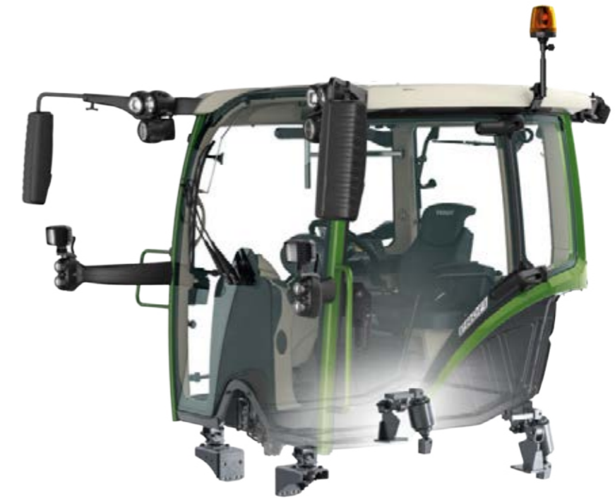
□ The super comfort seat has a seat heater, rotary adapter and pneumatic lumbar support - prerequisites for comfortable work during long shifts.
